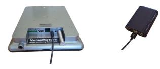
The LiveNoise Terminal has three spare USB ports. You can use any of these to connect to the Noise Sign.
